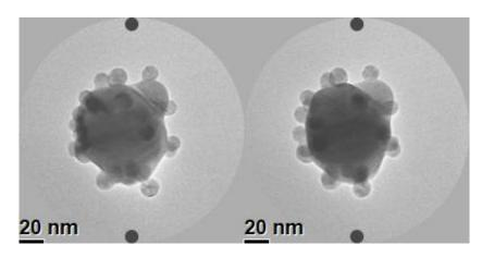
Figure 4: Stereo pair showing three connected Au particles decorated by smaller Au satellites. The difference in  $\alpha$ -tilt is 14.8°.
