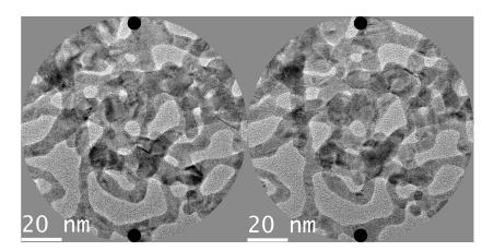
Figure 7: Stereo pair showing a debris of Au networks. The difference in  $\alpha$ -tilt is 14.9°.
