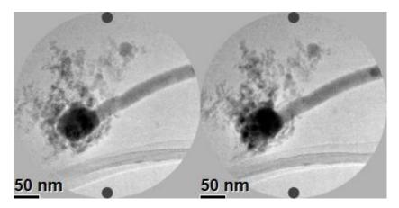
Figure 3: Stereo pair showing a BiRh nanowire growing from a round particle surrounded by the nebula of tiny stuff. The difference in  $\alpha$ -tilt is 20.4°.
