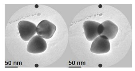
Figure 6: Stereo pair showing a agglomeration of three Au particles of nearly cubic shape. The difference in  $\alpha$ -tilt is 22.0°.
