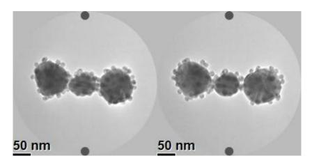
Figure 5: Stereo pair showing three connected Au particles decorated by smaller Au satellites. The difference in  $\alpha$ -tilt is 19.5°.
