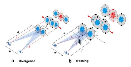
Figure 2: Two ways of viewing stereo pairs: (a) divergence of eyes and (b) crossing eyes. Blue rays represent "normal" view while red rays demonstrate how the viewing directions should be changed to provide 3D perception. Viewing beams for two eyes are shown by the red lines. In both viewing techniques, two images in a stereo pair are seen as a row of three images where the central image delivers stereo view.
